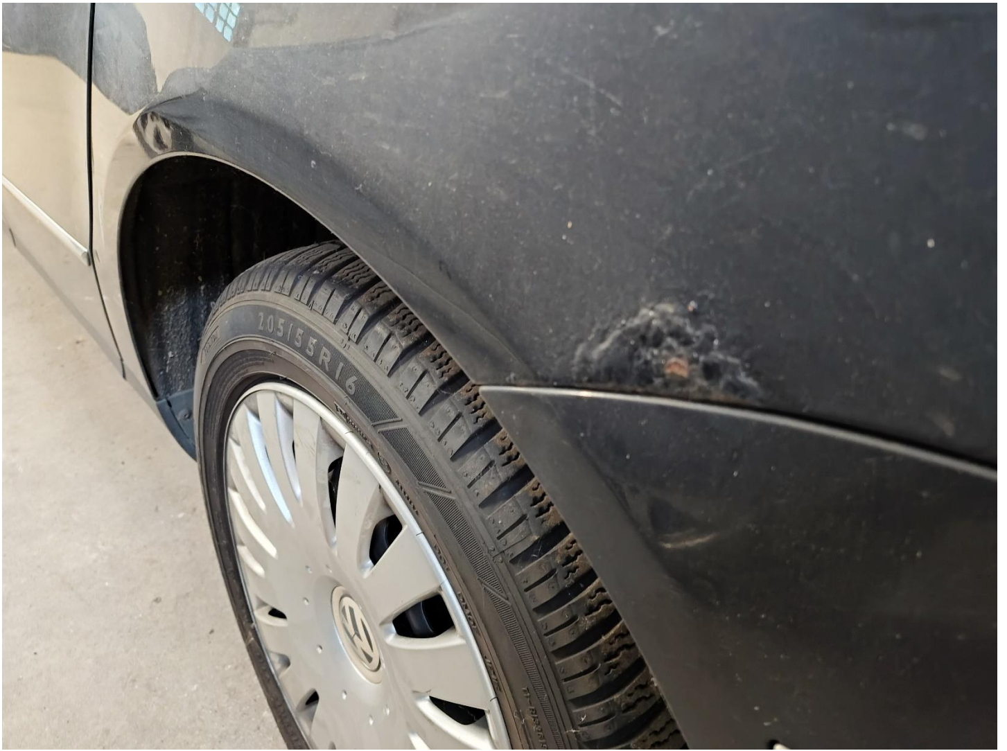
Korrosion + Delle hinten links
